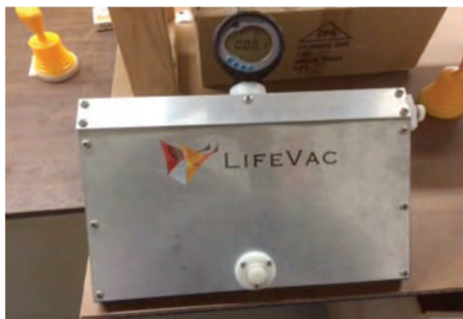
Figure 1. Vacuum testing fixture used in LifeVac testing.
